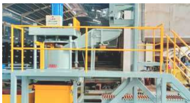
Oil Sludge Filter Press Machine separating oil and metal scrap for disposal
